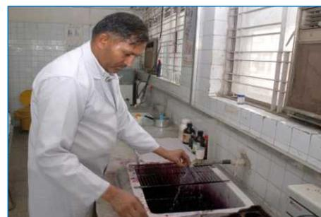
Figure 14. Gram's staining procedure (draining)
