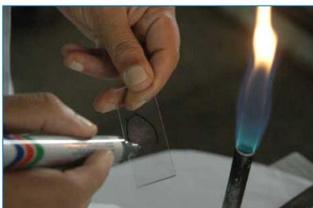
Let the slide dry completely in air. Label the slide with a glass maker pen/ pencil. (Fig.9)
