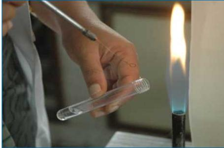
Take a portion of the specimen to be examined for pus, by placing the loop flat on the surface of the liquid. Fig. 5 & 6
